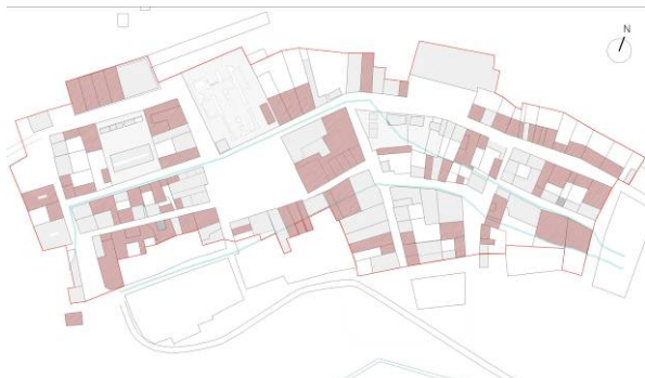
Figure 3: Plan of San Lorenzo de Tarapacá zoning by earthquake damages. The dark red sites are the ones for been re-built and the gray ones are those for been restored.
